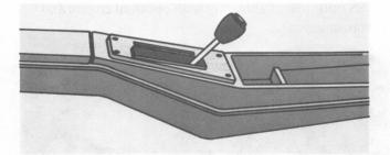
Console • Available for use with Strato-bucket option • Includes compartment for extra stowage
