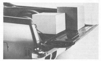
**Double-wall tailgate construction,** too. Designed for one-handed operation • Helps protect against cargo dents • Tailgate parks almost flush with cargo bed and nearly level • You hoist load only to box floor height, slide it smoothly inside.
