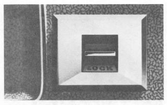
**Power door locks** • Touch a button to lock both doors • Individual controls located on each door.
