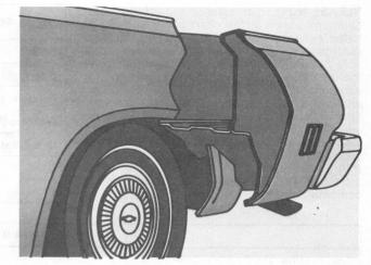
**Double-wall construction** helps protect exterior wall from inner wall cargo dents • Doors, hood and roof also made of two sheets of steel • Every fender has an inner fender to help protect against the effects of water, salt and road dirt • Large rear fenders offer protection against road splash.
