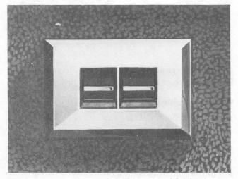
**Power windows** • Driver has control for both windows located on door • Separate control for right-hand window on passenger door.
