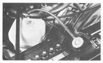
**Standard coolant recovery** system on El Camino collects and returns radiator overflow.
