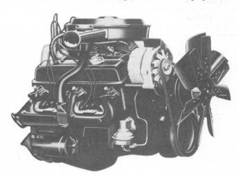
**305-2 V8** • Now the base engine on V8 models except in California • Has smaller cubic-inch displacement than the engine it replaces, but shares all the big-engine features that contribute to good performance and efficient operation using no-lead fuel.
